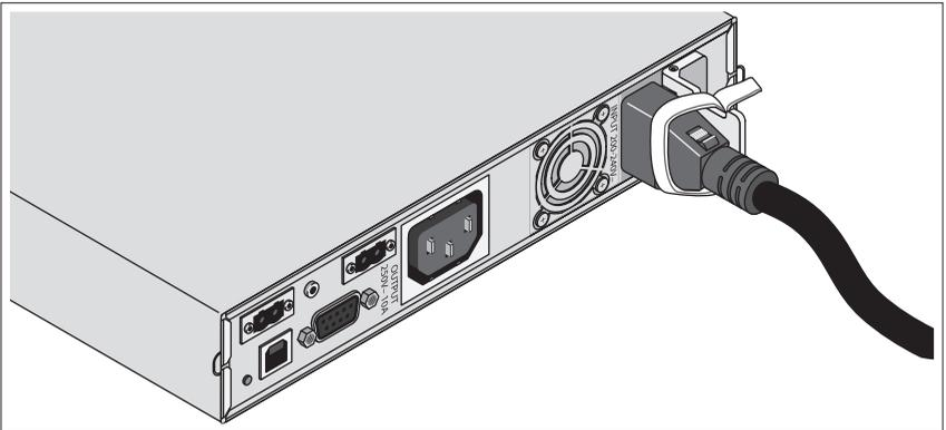
Secure the power cable connected to the BPS as shown in the illustration.
