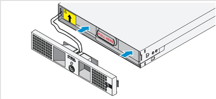
Align the battery with the power module and reinsert the battery. Ensure that the battery is fully seated in the power module. If the battery is not fully inserted into the power module, the battery front cover will not close properly.
