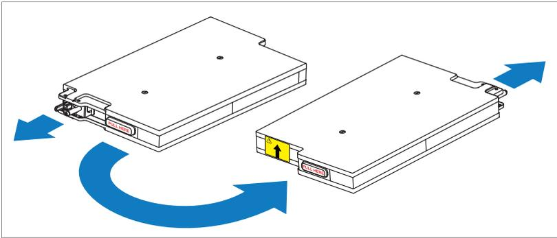
Rotate the battery 180° so the blind mate connector faces toward the back of the power module chassis.
