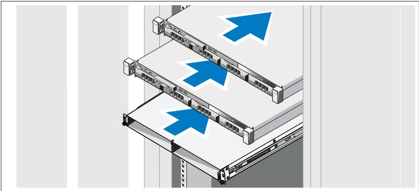
Assemble the rails and install the system and backup power supply (BPS) in the rack. Follow the safety instructions and the rack installation instructions provided with the solution.
