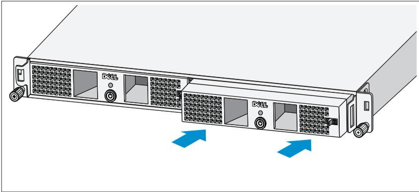
Insert the power modules into the chassis module bay with the back panels toward the back of the chassis.
