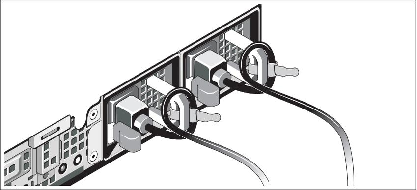
Bend the system power cable(s) into a loop as shown in the illustration and secure the cables to the brackets using the provided strap. Plug the other end of one power cable to a grounded electrical outlet and the other cable to the BPS. For more information, see "Cabling the Solution" on page 9.
